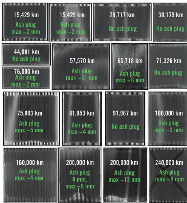
FIGURE 4 CT scan images of GPFs tested on public road over different mileage (note: scale is different for the images) © Corning
